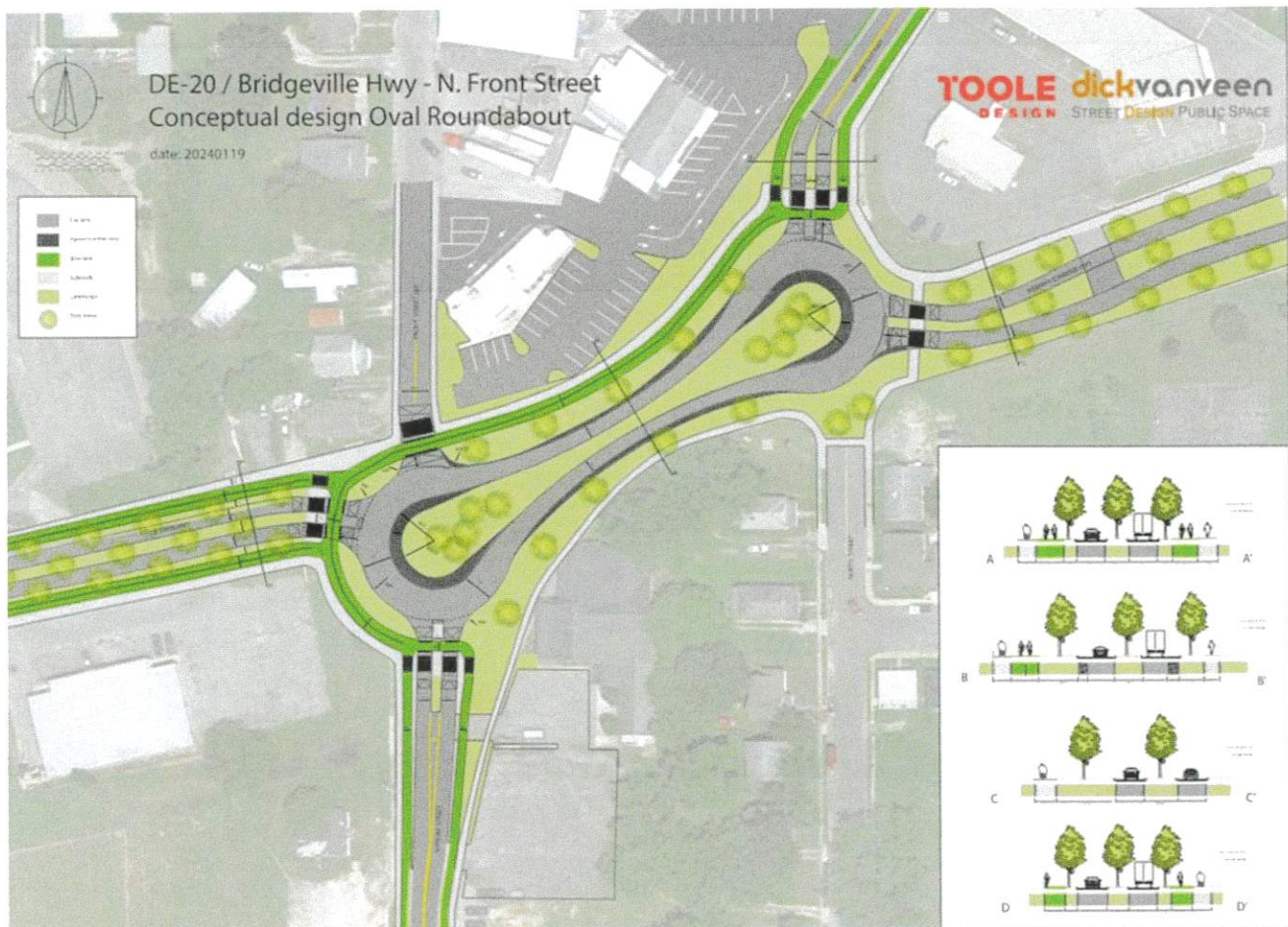
Figure 5 Proposed Conceptual Design for Roundabout
